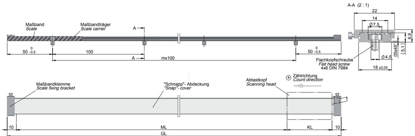
$GL = (m + 1) \times 100$  [mm]      $m = 1, 2, 3, \dots, 29$
