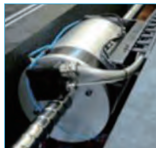
牵引电机, 60kW (MACCON)
